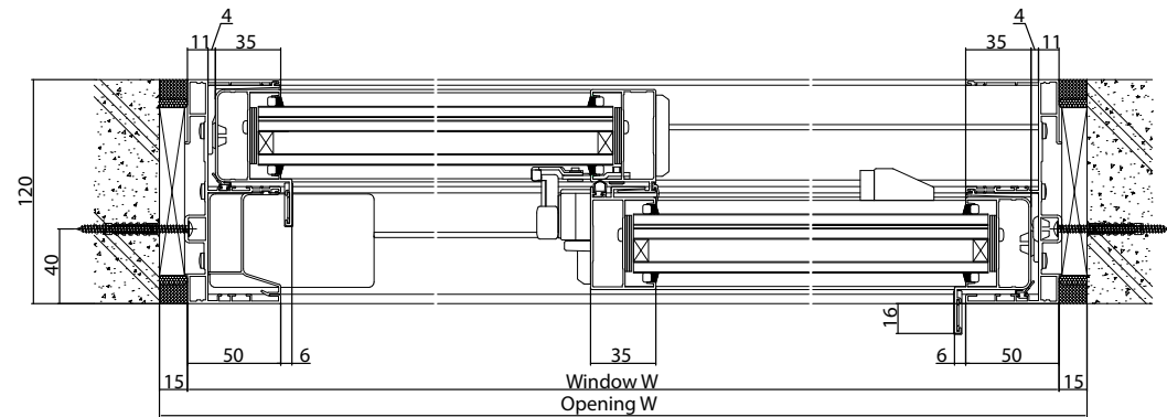
Horizontal section: Sliding window (2 panels on 2 tracks)
